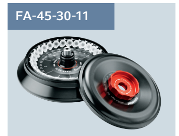
30 x 1.5/2 mL micro tube rotor with aerosol-tight lid for safe centrifugation of hazardous samples. Max. speed 20,800 x g (14,000 rpm).
