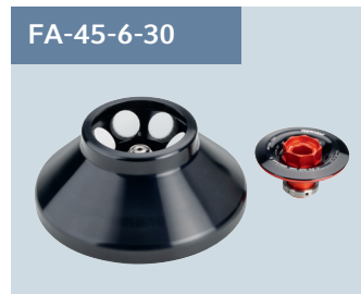
6 x 50 mL conical tube rotor with aerosol-tight QuickLock lid for tubes from 5–50 mL. Max. speed 16,639 x g (11,000 rpm).
